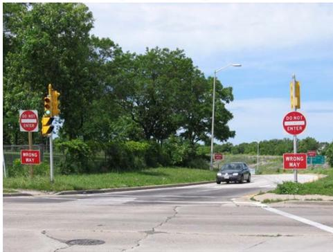
The Wisconsin Department of Transportation (WisDOT) has implemented a variety of wrong way driving (WWD) countermeasures throughout the Milwaukee metropolitan area due to an increase of WWDs during the hours of 11 p.m. and 6 a.m. These countermeasures include: detection equipment, red reflective tape, doubling up and lowering signs, and pavement markings. Between 2012 and 2015, 336 WWDs were reported, with 123 unconfirmed and 152 confirmed.
